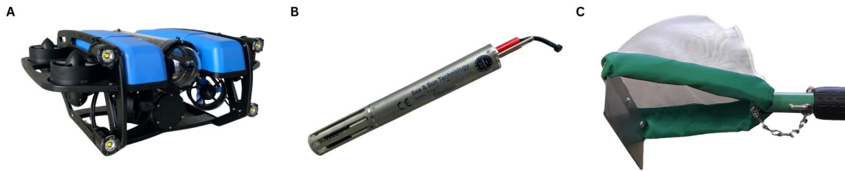
Fig. 3 Sampling devices: Remotely operated vehicle (ROV) (A), CTD probe (B), and pile scraper (C).
