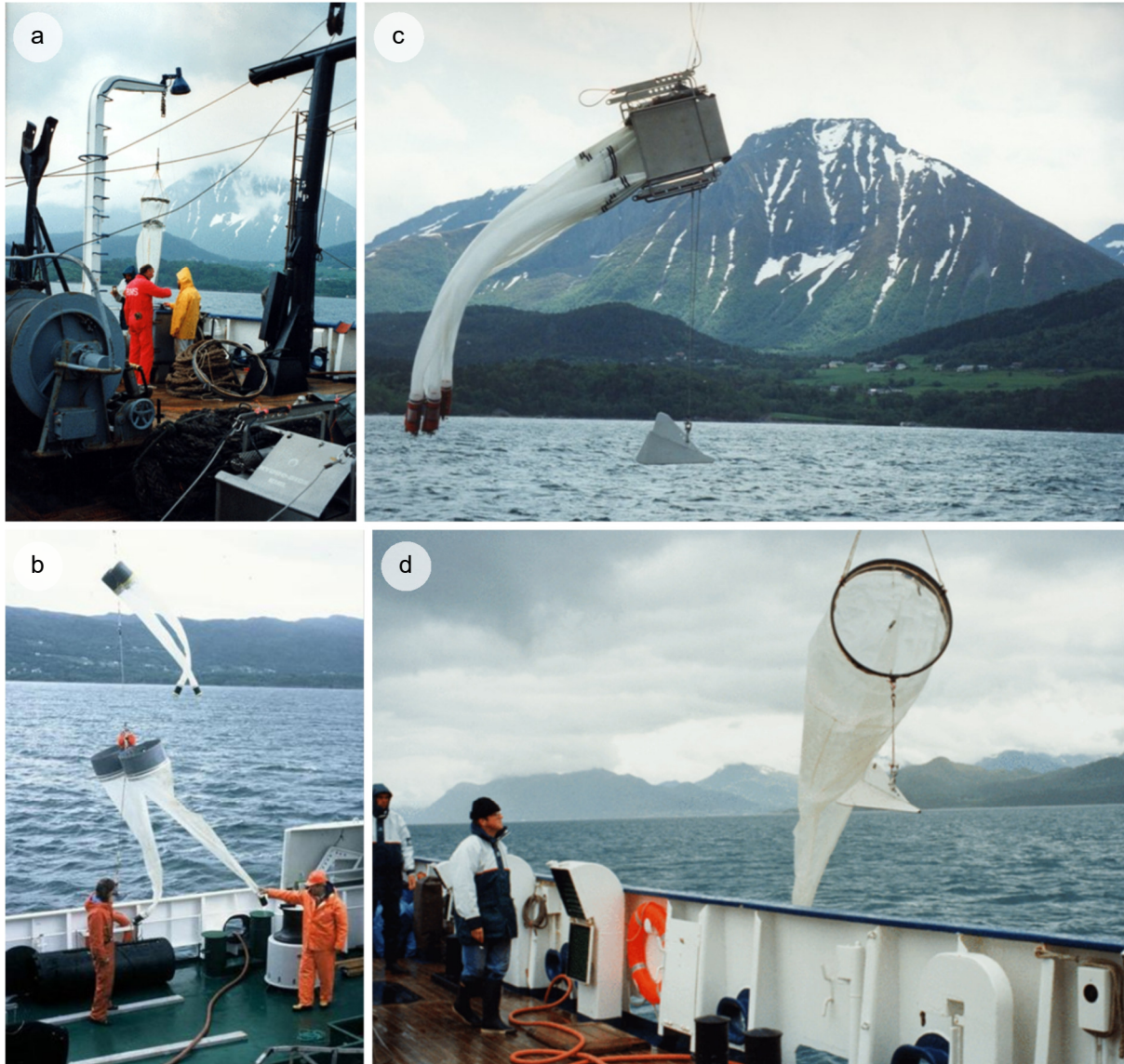
Figure 3.1: a, The WP-2 UNESCO Standard net being deployed aboard the R/V A. v. Humboldt; b, Twenty cm and 60 cm Bongo nets ready for deployment from the R/V Johan Hjort; c, The Multinet rigged for horizontal towing from aboard the R/V A. v. Humboldt; d, Deployment of a CalCOFI net from the R/V A. v. Humboldt. All photos stem from an ICES/GLOBEC Sea-going workshop for inter-calibration of plankton samplers at Storfjorden, Norway, June 1993 (ICES, 2002) (after Telesh et al., 2009).
