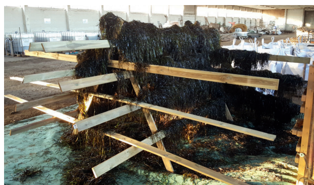
Figure 1.11 Passive (pre-) drying on a wooden structure at the Hanseatische Umwelt CAM GmbH facilities, July 2020)
