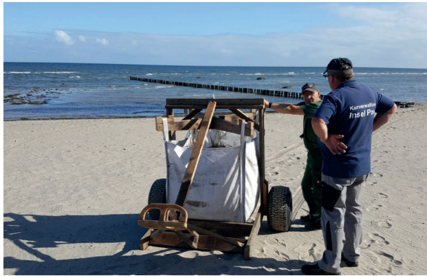
Figure 1.6 A big-bag trolley for transportation of eelgrass manually collected with a stone fork (Island of Poel, Germany, July 2020)
