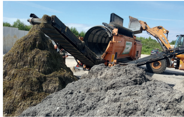
Figure 1.7 Screening of the beach wrack at the temporary storage facility at Boltenhagen, Germany, July 2020
