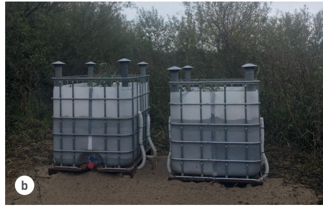
Figure 6.10. Constructed pilot plant of RBS at WWTP in Swarzewo: (a) reed in the RBS (August 2020), (b) two cubic pilot plant RBS (October 2019), photo: A. Kupczyk
