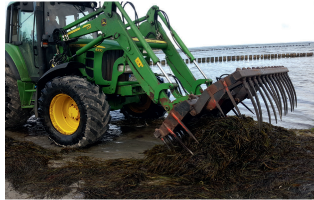
Figure 1.5 Beach wrack collection in the splash zone using a tractor with a pitchfork and a rake (Island of Poel, Germany, July 2020)
