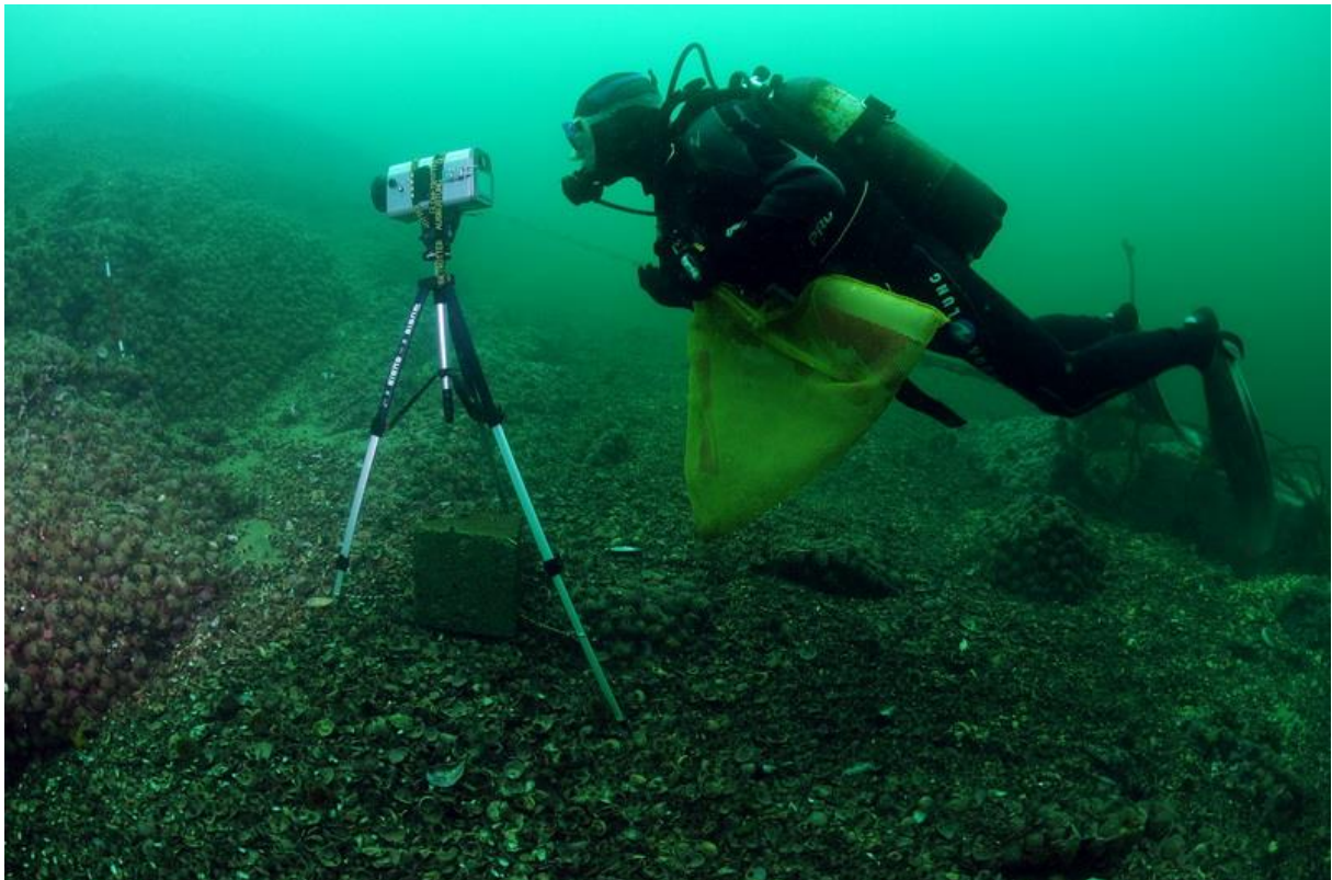
Fig. 2: Installation of a SONY TVR 995 video camera near Caleta la Arena, Reloncaví Fjord, 10 m depth
