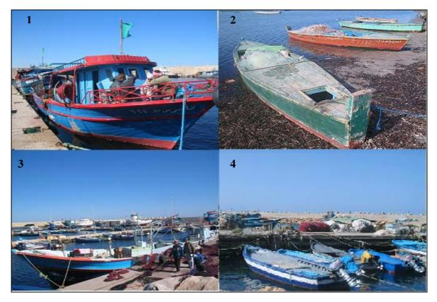
**Fig. 2**. The fishing vessels used along the Libyan coast: 1 Mator, 2 Batah, 3 Lampara, 4 Flouka.
