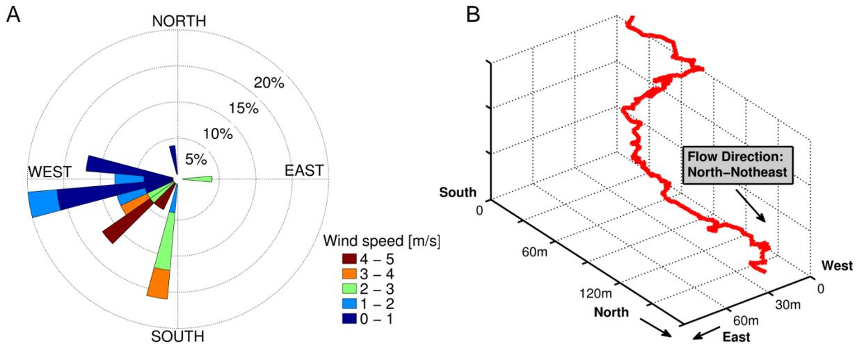
**Fig. 7:** (A) Wind rose for the second tracer study. (B) Simulated flow path of a particle using the XYZ velocity components of the acoustic Doppler velocimeter at the starting point of the tracer study (path over 24 hours: 2014-08-12 noon until 2014-08-13 noon).
