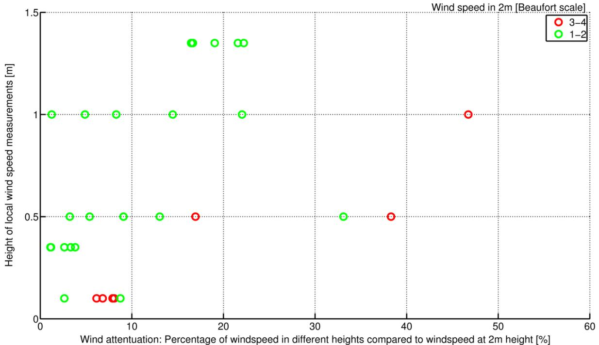
**Fig. 5:** Wind attenuation profiles recorded within the reed bed. Wind speeds (averages over 1 hour) in 2m height were compared to wind speeds at different heights between 10 and 135cm inside the reed bed ( $n = 29$  hours of wind data during 11 days).
